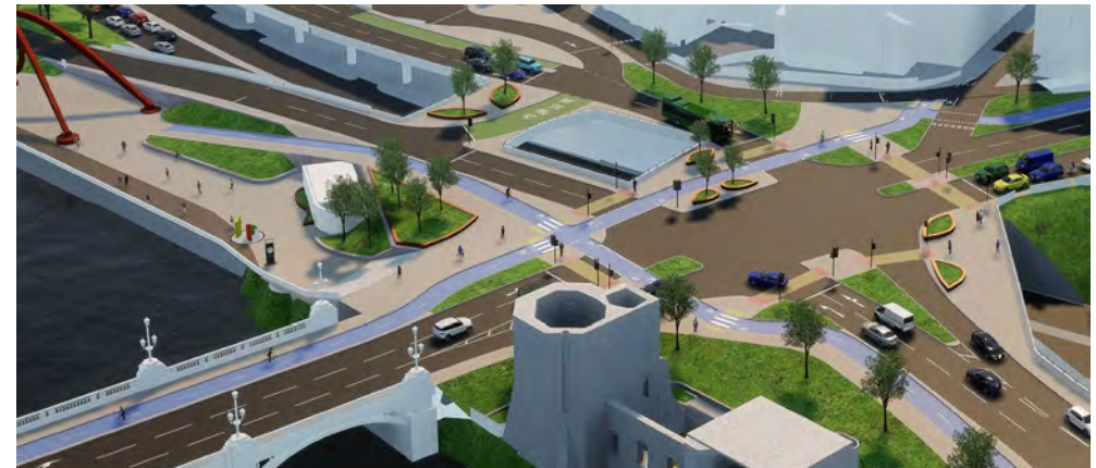
More direct, surface level walking and cycling routes through the reconfigured junction. Buses will benefit from priority, reducing delay.
